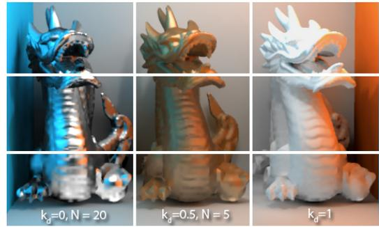
**Figure 10:** Final gathering at every pixel (0.83 Hz, top),  $1/4$  of all pixels (2.2 Hz, middle), and  $1/16$  (4.2 Hz, bottom). Preview quality can be achieved with a very low number of gather samples for diffuse or low-glossy materials.
