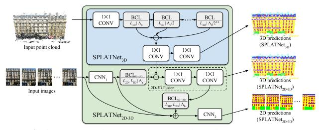
Figure 3: SPLATNet. Illustration of inputs, outputs and network architectures for SPLATNet<sub>3D</sub> and SPLATNet<sub>2D-3D</sub>.
