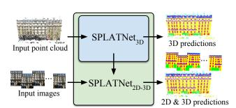
Figure 1: From point clouds and images to semantics. SPLATNet<sub>3D</sub> directly takes point cloud as input and predicts labels for each point. SPLATNet<sub>2D-3D</sub>, on the other hand, jointly processes both point cloud and the corresponding multi-view images for better 2D and 3D predictions.
