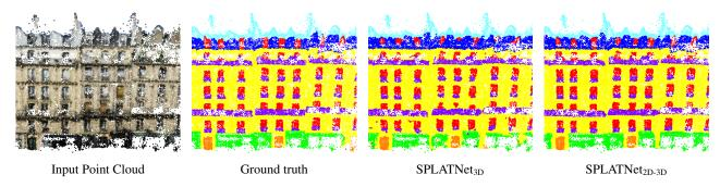
Figure 6: Facade point cloud labeling. Sample visual results of SPLATNet<sub>3D</sub> and SPLATNet<sub>2D-3D</sub>.
