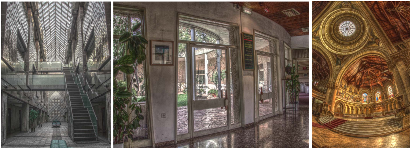
Figure 17: We stressed our approach by applying a strong range compression coupled with a large detail increase ( \alpha = 0.25 , \beta = 0 , \sigma_r = \log(2.5) ). The results are dominated by local contrast and are reminiscent of the popular, exaggerated “HDR look” but without the unsightly halos associated with it. In terms of image quality, our results remain artifact-free in most cases. We explore further parameter variations in the supplemental material.
