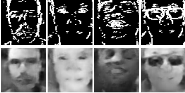
Figure 8: Intensity reconstruction result inferred by the network described in Section 3.2 and trained on the WIDER simulated data. The top row shows 64x64 face crops captured with the prototype camera, the bottom the corresponding reconstructed images. While the quality is not quite on par with the intensity reconstructions, it has to be noted that the resolution of the crops in Figure 5, is 96x96, i.e. 1.5x larger.
