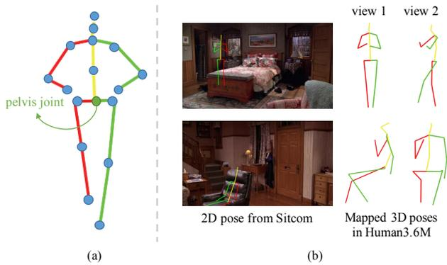
Figure 8. (a) We represent each pose using the coordinates of 17 joints. We represent the pose location using the coordinates of the pelvis joint (green dot). (b) We map each 2D pose from [27] to a 3D pose in the Human3.6M dataset [12]. The last two columns show corresponding 3D pose of the 2D pose in column 1 visualized from two different views.
