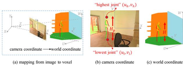
Figure 9. (a) Mapping from pixel coordinate system to world coordinate system. (b) Illustrations of human height  $H_p$  in pixel coordinates, “highest joint” and “lowest joint” in the pose. (c) Illustrations of human height in world coordinate system.
