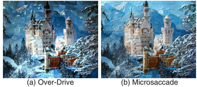
Fig. 2. Prototype problems due to transmissive modulations. (a) Photograph of nonlinear color blending due to over-driving liquid crystals. (b) Sharp block boundaries perceived during microsaccade.
