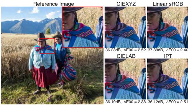
Fig. 6. Comparing simulated results optimized in different color spaces. Optimizations done in the linear spaces give higher PSNR, but the perceptual optimizers give better  $\Delta E_{00}$  values. Although the linear sRGB optimizer gives good result, its framework in practice does not allow the matching of the color filter spectrum in Eq. 2. Image courtesy of Jiamin Bai.
