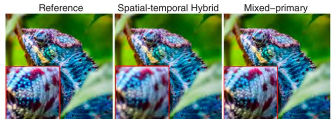
Fig. 9. The simulated spatio-temporal hybrid approach reproduces the complete color gamut by showing red and green colors in the first frame and blue in the second frame. Since the reds and greens are spatially interleaved (checkerboard), the maximum spatial resolution is not as high as in our mixed-primary approach. Image courtesy of Flickr user kuhnmi.
